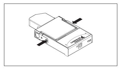
Figure 5. Locking Module into Place
